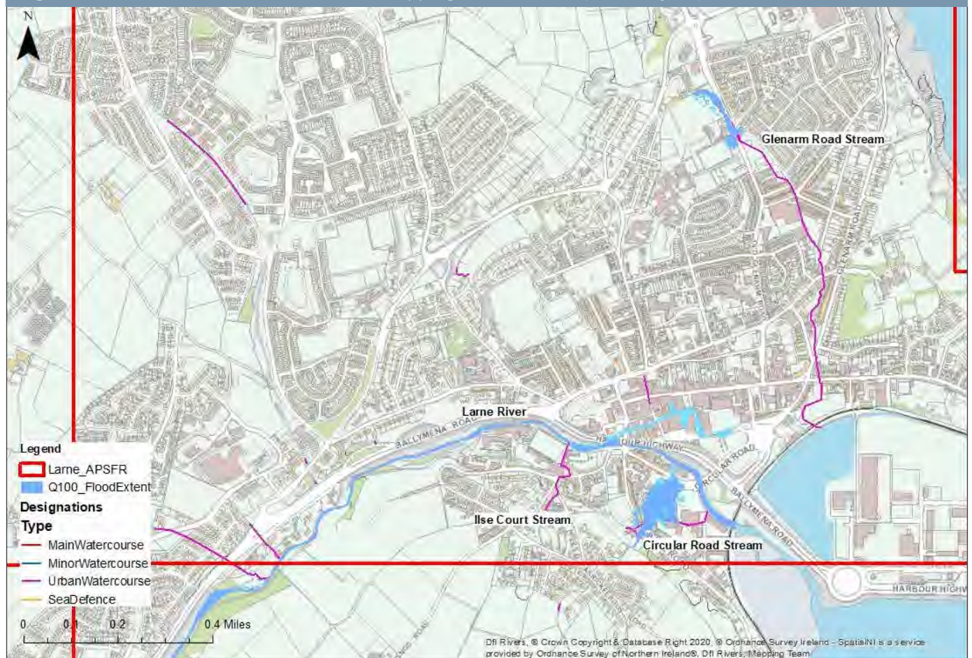
Figure 5.6-9: Overview of fluvial hazard mapping for a 1 % AEP (1 in 100 year) flood event
