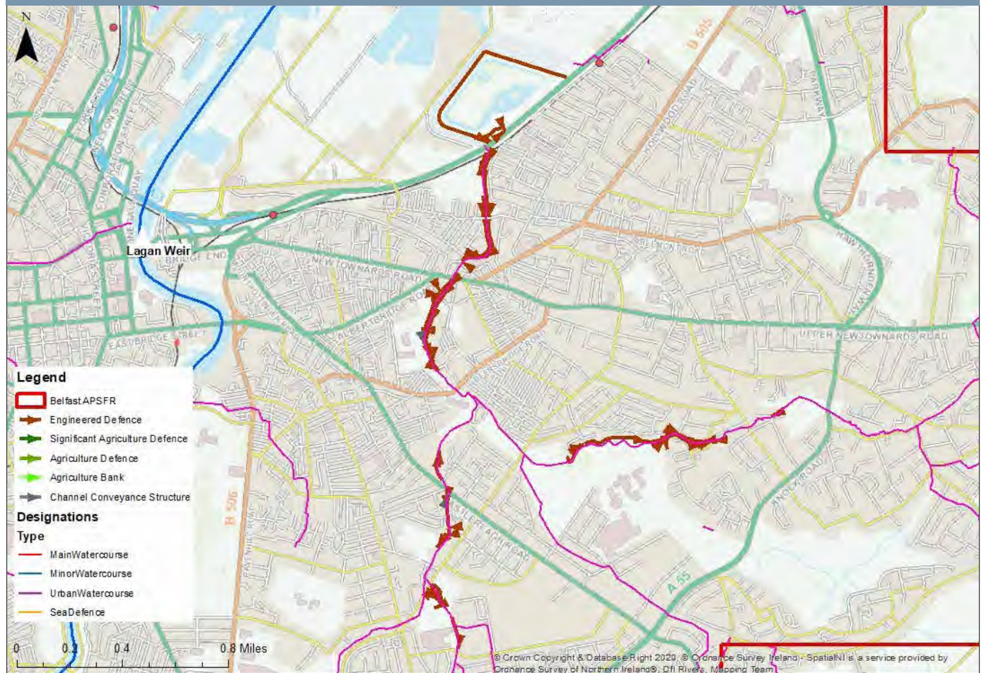
Figure 5.1-12: Flood defences in the eastern section of the Belfast APSFR
