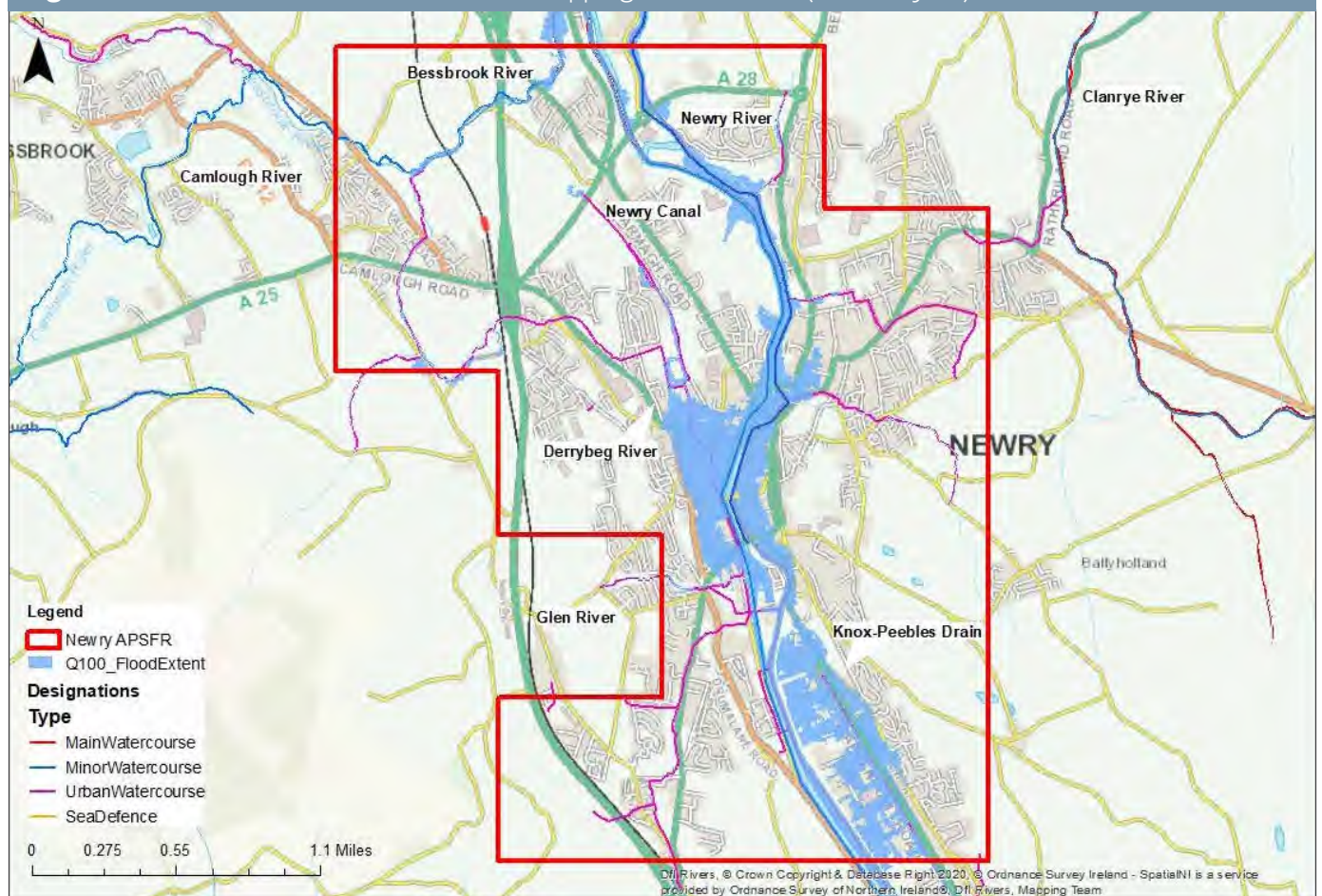
Figure 5.3-10: Overview of fluvial hazard mapping for a 1 % AEP (1 in 100 year) flood event
